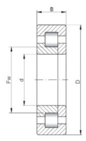
460 mm x 620 mm x 95 mm ISO NUP2992 cylindrical roller bearings
