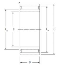
NAO45X72X20 Bearing 2D drawings and 3D CAD models
